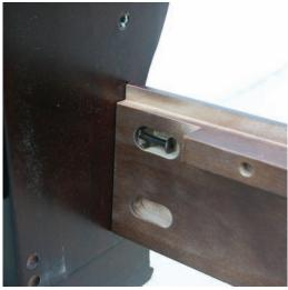
STEP 6: Place bolt into hole and fasten it to the headboard. If clip is falling out, it is installed incorrectly. Please refer to step 5. Repeat for bottom hole. Tighten as needed.
